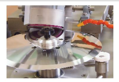
The PRIMEdge ALC-600 Circular Blade Sharpener is especially designed for the meat processing industry and offers models for large processing facilities down to small locker plants. With a unique blade rotation system, the ALC-600 offers complete control of the sharpening operation, which brings you the desired bevel angle and flatness every time.
